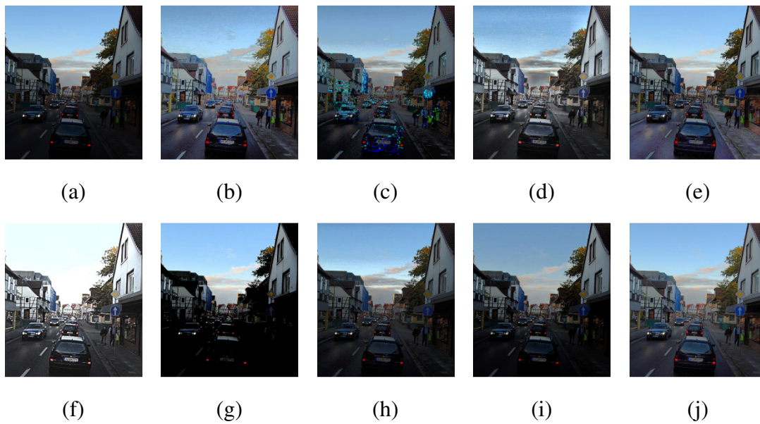
Figure 2: (a) Original Image; Enhanced Images by (b) HE, (c) BPDHE, (d) CLAHE, (e) NPEA, (f) BGupta2017, (g) Pal1980, (h) BPDFHE, (i) Hanamandlu2016 and (j) Proposed Method
